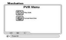
Format Hard Disk: After fitting Hard Disk or to erase previously recorded events, press OK on this menu. A message Formatting will erase all data will come up. To format press OK.
